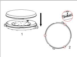
7. Re-fit the diffuser by placing it over the base and lock into position using the screws.
