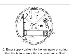
that the hole is smooth or a grommet is fitted and connect it to the terminal block (see wiring instructions).
