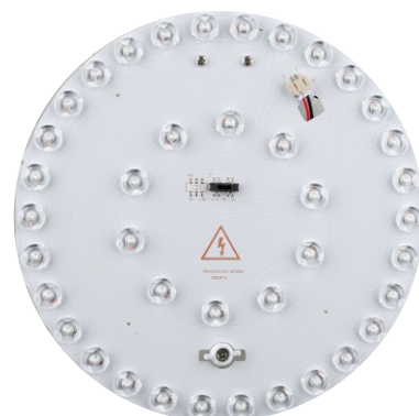
Evenly spread LED chips for a uniform light distribution
