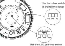
Use the LED gear tray switch to change the CCT temperature
