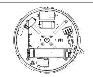
5. Enter supply cable into the luminaire ensuring that the hole is smooth or a grommet is fitted and connect it to the terminal block (see wiring instructions).
