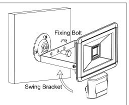
Install the swing bracket onto the base using the fixing bolt
