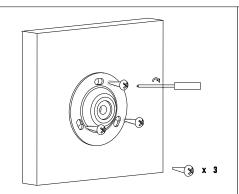
Mount the round bracket on the wall using the three fixing bolts
