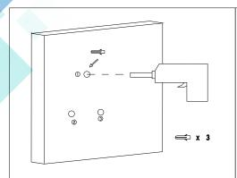
Mark the position, drill the holes and install the wall plugs
