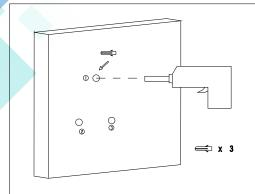
Mark the position, drill the holes and install the wall plugs
