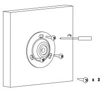
Mount the round bracket on the wall using the three fixing bolts
