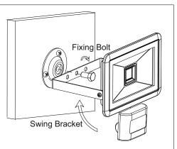
Install the swing bracket onto the base using the fixing bolt
