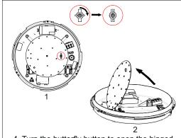
4. Turn the butterfly button to open the hinged gear tray to allow access to the connections.
