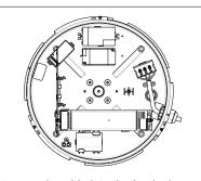
5. Enter supply cable into the luminaire ensuring that the hole is smooth or a grommet is fitted and connect it to the terminal block (see wiring instructions).
