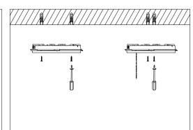
6. Position and fix the base to a suitable solid surface using suitable fixings and close the hinged LED gear tray
