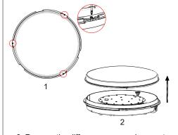
3. Remove the diffuser screws and separate it from the base.
