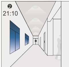
2 21:10 Light dims to stand-by level after the hold time.
