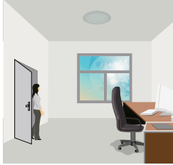
1. Off With enough natural light the PIR will not trigger when presence is detected.
