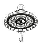
2. Install the sensor on the sensor base and tighten it.
