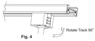
5. Track heads may be positioned anywhere along the track length. Aim the fixture to your desired position. Fixture adjusts 350° horizontal and 180° vertical.
