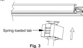
4. Rotate the track adapter 90°. The arrows should point to the grooved side of the track (**Fig. 4**). Make sure the locking tab seats in the track slot.
