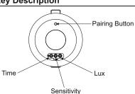
Step 1: Press and hold the pairing button on the PIR sensor for 3 seconds; the green LED indicator light will flash slowly (once per second) and then release the button.
