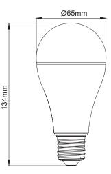
Direct replacement for A65 GLS lams GREATER LIGHT OUTPUT THAN EQUIVALENT 150W INCANDESCENT LAMP
