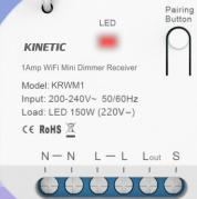
Input: 200-240V~ 50/60H Load: LED 150W (220V~)
