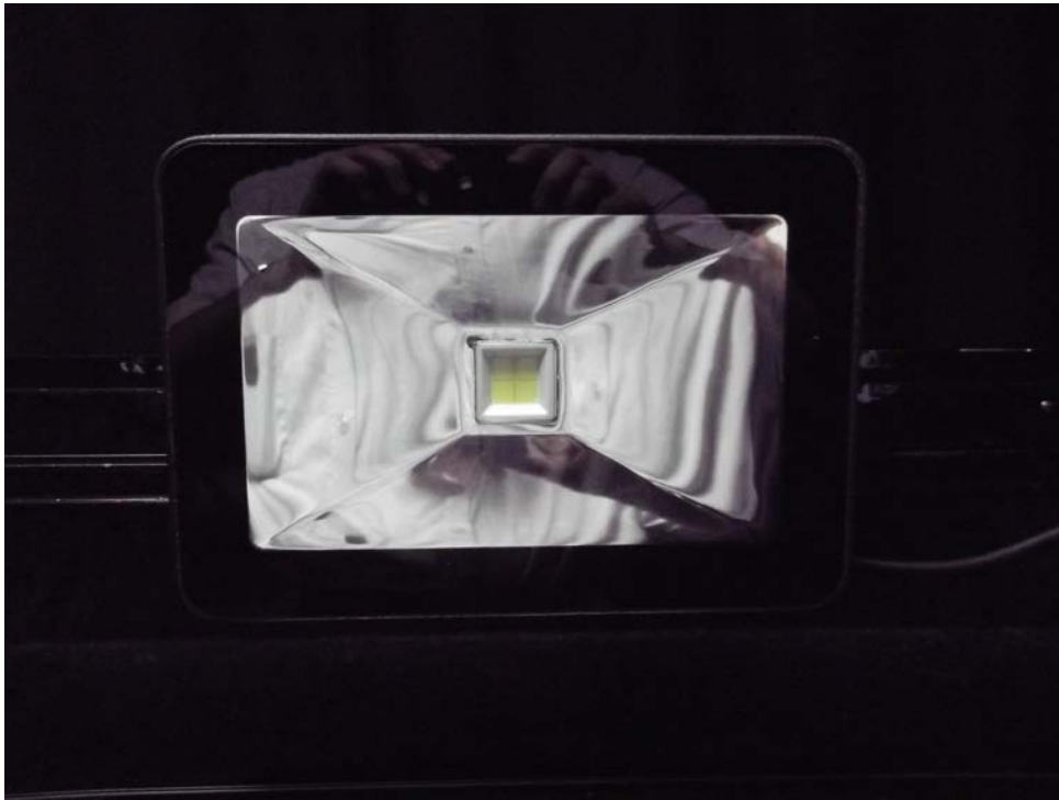
Photo 1: Luminaire on goniometer mount
