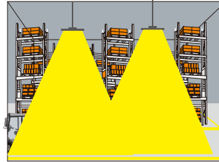
After hold time, the lamp dims to a low light level if no new motion trigger.
