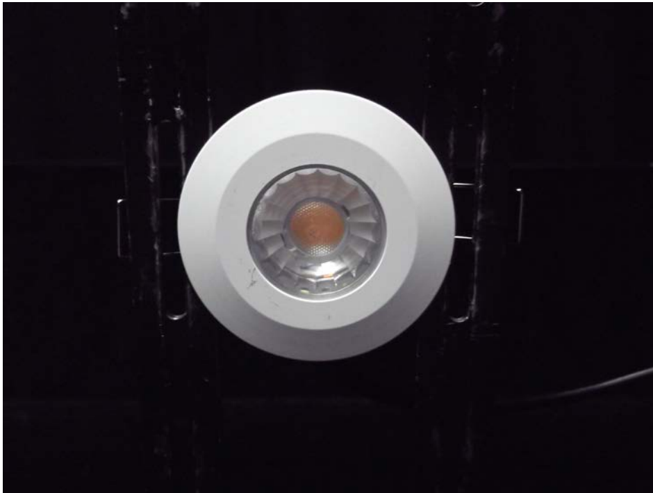
Photo 1: Luminaire on goniometer mount
