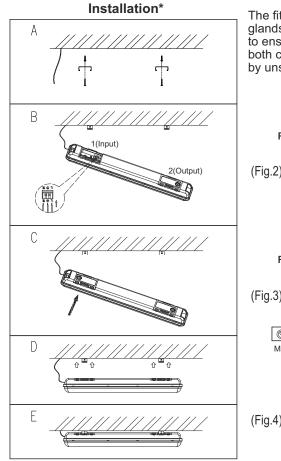
The fitting comes with both waterproof cable glands installed, one side has a silicone cover to ensure the IP65 rating. In order to utilize both connections, remove the blanking plate by unscrewing the cover.
