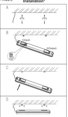
For detailed wiring instructions see Fig. 2 (input) and Fig. 3 (output) on the next page.
