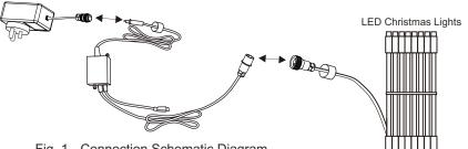
Fig. 1 - Connection Schematic Diagram
