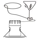
Fold spring clips upwards and insert fitting into hole
